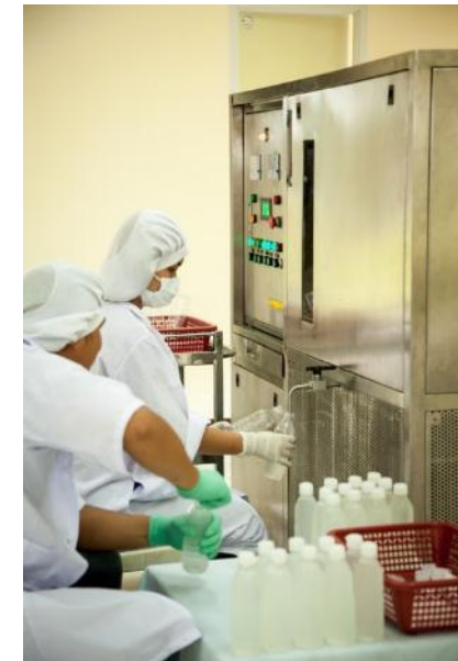
Coconut water pasteuriser and chiller
